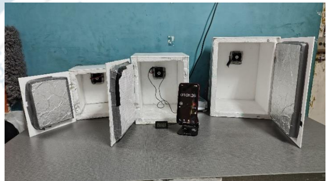
Fig. 4. Test Setup of Refrigerator
