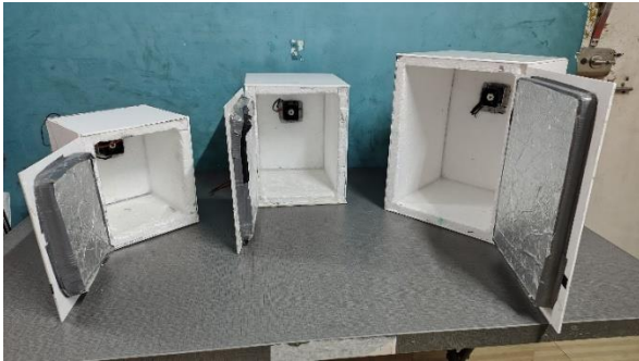
Fig. 3. Assembly of Peltier Module in Refrigerator
